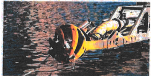
Plastic bag trash in the Woonasquatucket and Providence Rivers tangled in dredge machinery and increased the time and cost to dredge the rivers.
